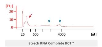
Blood samples were drawn into EDTA (legacy) tubes or Streck RNA Complete BCT, mixed following IFU, and plasma isolated. Total nucleic acid was purified, DNase-digested, concentrated, and then run on the Agilent Bioanalyzer using the RNA 6000 Pico Kit. The blue arrows indicate larger 18S and 28S ribosomal RNA peaks while the red arrows denote smaller and highly fragmented RNA species.
